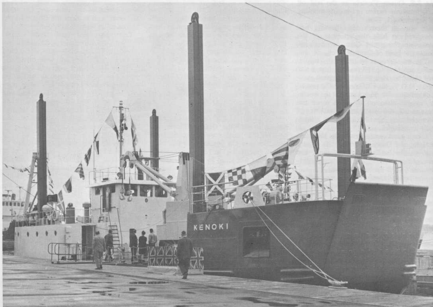
LONG-LEGGED SHIP —The Canadian Coast Guard's newest ship, christened CCGS " Kenoki " at Prescott, Ont., on Saturday, August 15, can stand on her own feet when necessary. The unique vessel, seen here at the Prescott Marine Agency, is designed to serve as an agency tender and, when working at marine construction projects, can lower her "legs", or spuds as they are properly termed, to the bottom in order to remain stationary where the waters are shallow and the current swift.
