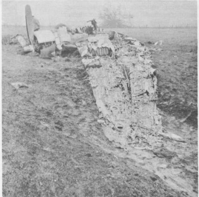
The investigators found the left wing of the DC4 with No. 1 engine still hanging on. The wing was completely burned, but they were able to determine that it was upright when it struck the ground and that the propellor had been feathered.
