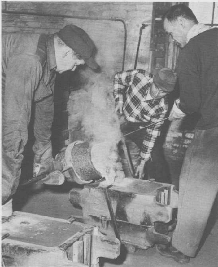
Left: Casting a whistle valve for a buoy. Prescott employees (left to right) Gerald Kennedy, Frank Cipra and Donald Smith pour melted brass from a red-hot crucible into molds. This job requires proper timing and a keen awareness of safety procedures. (The men are protected by steel-capped shoes and asbestos leggings and gloves.)
