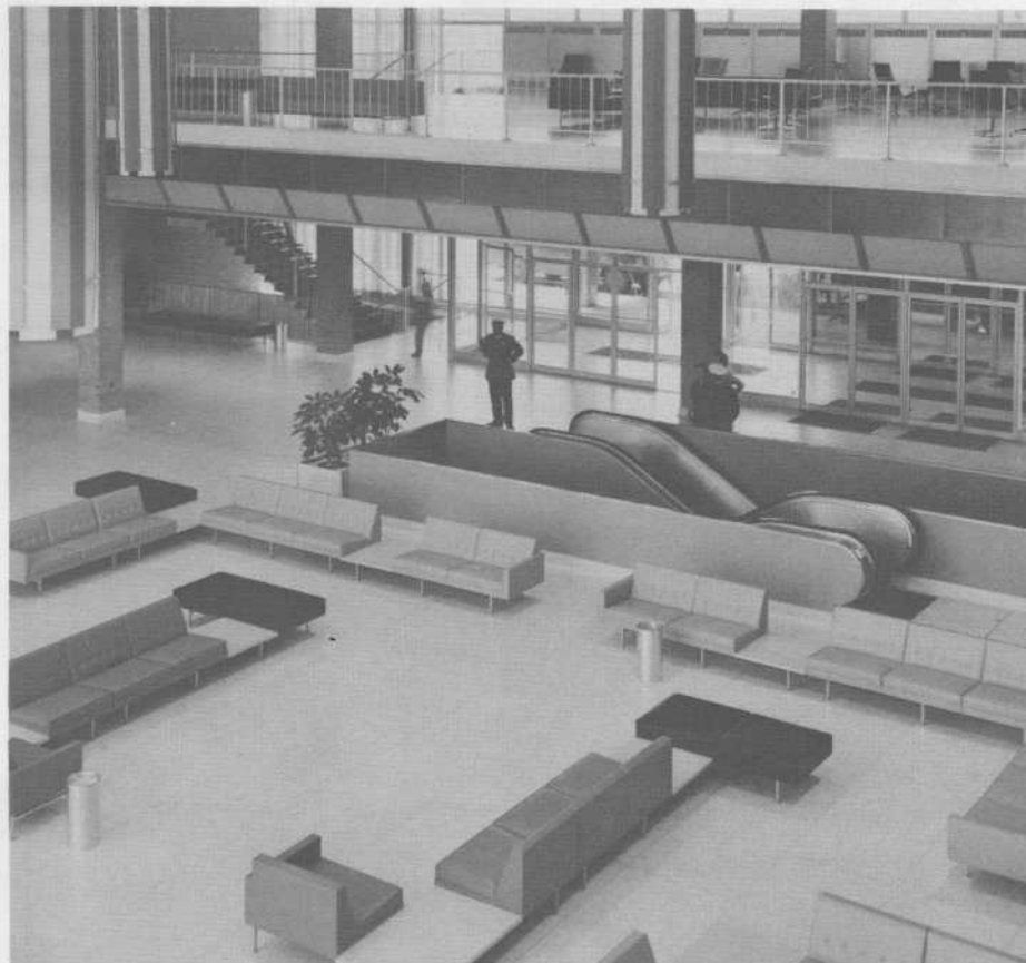
An ultra modern touch has been added to the new air terminal buildings through the extensive use of stainless steel and aluminum. In this view of the Halifax terminal these products have been used for door and window frames, stairway railings, furniture legs and cylindrical ashtrays.
