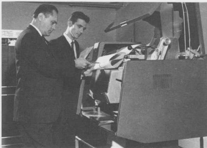
Data Processing Manager Don Burgess (left) and Programmer Gerald St. Amour check out a "memory dump" on the high speed printer to see if instructions relating to a program assembly are correct. This printer, as well as providing accuracy checks, produces the answers or results to the problems fed into the computer.
