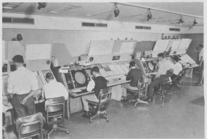
Area traffic controllers in darkened radar room keep track of all aircraft in vicinity on radar and by direct interphone to other centres.
